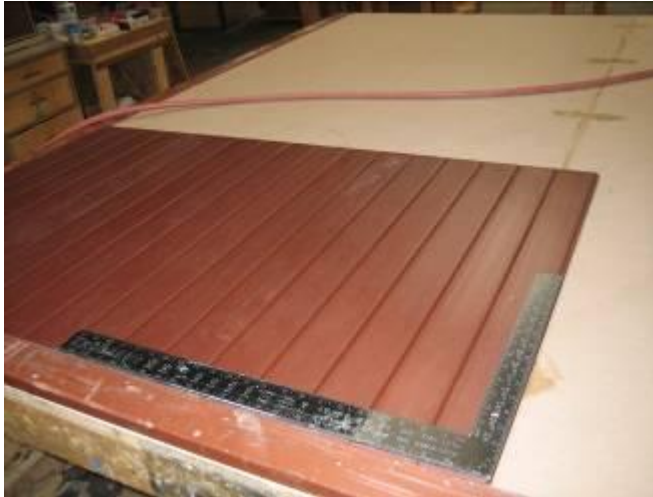
Image 4: Checking the T&G is square and tightly assembled
